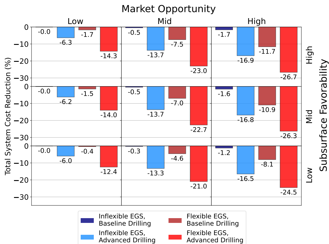
Figure 4: System cost reductions due to EGS deployment. Percentage difference in total annual cost between fully-decarbonized systems with and without EGS available, for the same set of scenarios shown in Figure 2.
